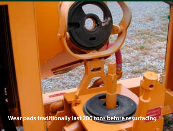
Simple Piccola Clamping System
