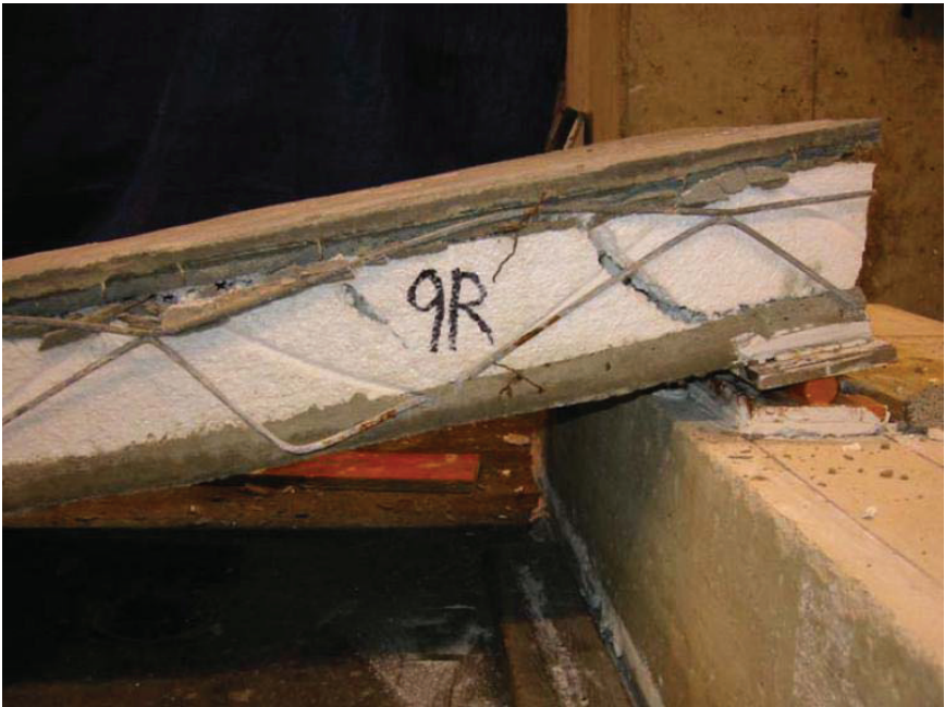
Figure 11 — Failure of panel number 9R.
