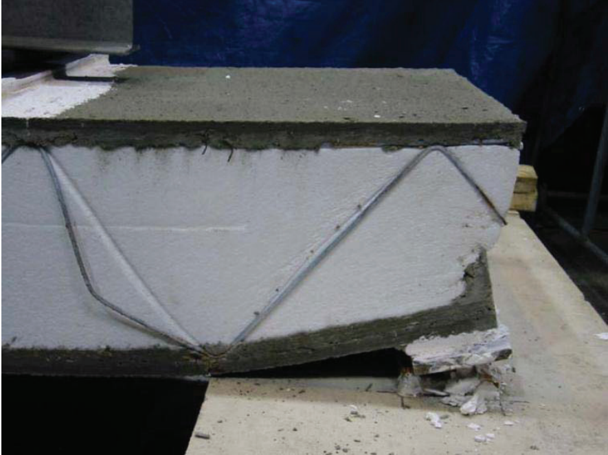
Figure 10 — Failure of panel number 4R.
