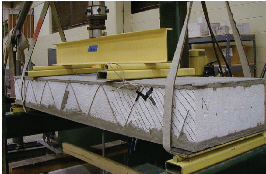
Figure 6 — Flexural test setup.
