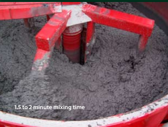
High torque mixing up to 2200 lbs per batch
